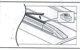
USE T-NUT M6X1.0 FROM F-KIT BAG FOR INSTALL AEROKLAS CROSS BAR IN SLOT ROOF RAIL ( REMOVE RUBBER SEAL BEFORE INSTALL ).
