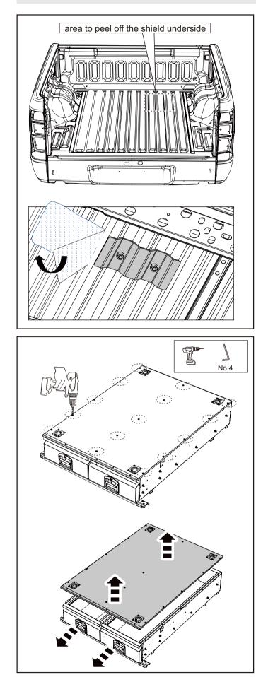
1. Prepare the vehicle for installation: - Remove Bed liner
