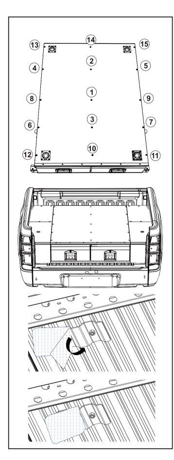
24. Re-attach the top panel assembly using the following tightening sequence shown. And fridges slide (if applicable).
