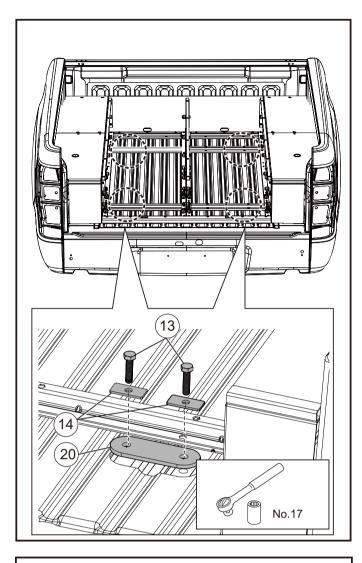
21. Lift drawer chassis assembly back into the vehicle tub and reinstall side contour panels. Align the frame back to the centre of the tub as per Step 5.
