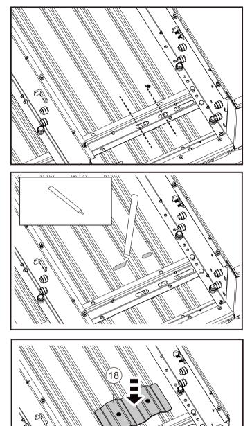
6. Mark drilling positions through the cross-member frame holes/slots The drilling positions on the left and right sides should fall on the center of the tub peak ridges in the floor.
