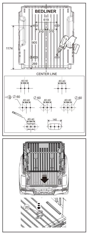
19. Make 4 slots (by holesaw diameter 60 mm. and cutter)
