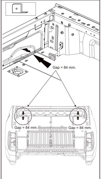
5. Place the drawer chassis assembly in the vehicle This step is critical to ensure that the unit is aligned & centralized in the tub against the contour panels, Position the unit to allow drilling points to be marked. it is critical that the unit is:
